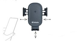
c. Touch the left or right button (or both) and place your phone in the car charger. Extend the adjustable foot to align the charging center should your phone not charge immediately.
